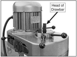
**Figure 42.** Drawbar loaded (Model G0747 shown).
